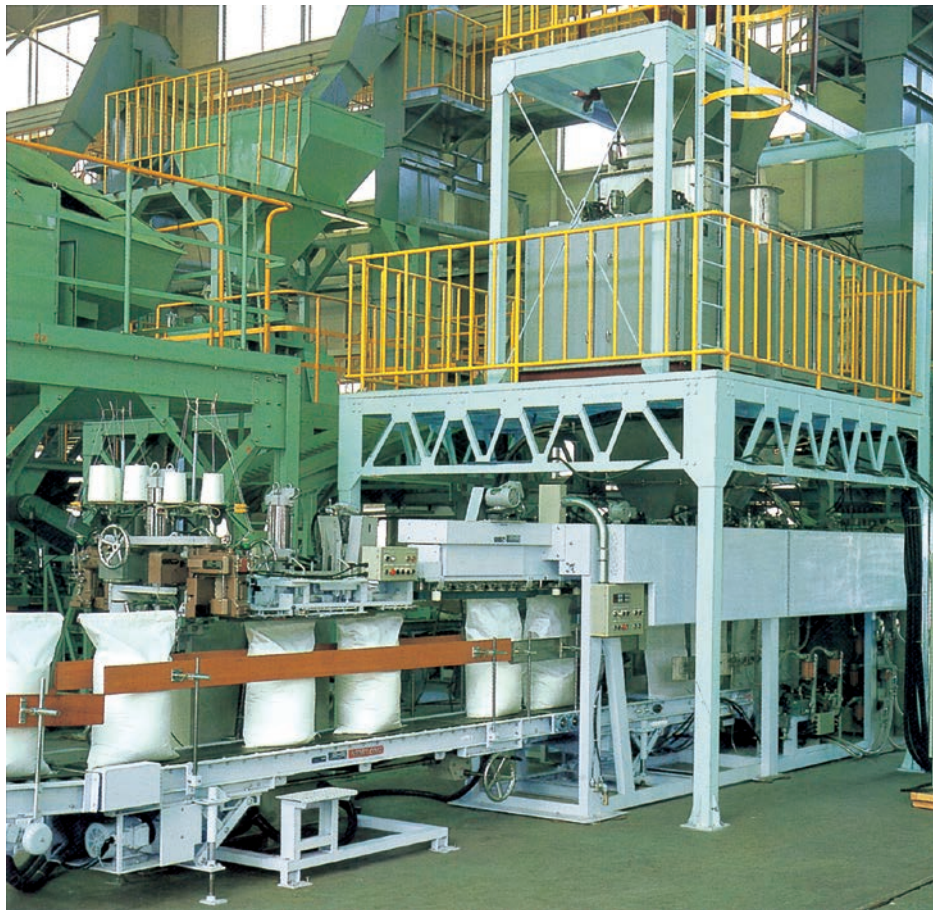
The photo shows Model 3CM-PD for bagging 40kg urea, using wovencloth bag. Two Duplex-scale installed overhead for a shop test.
